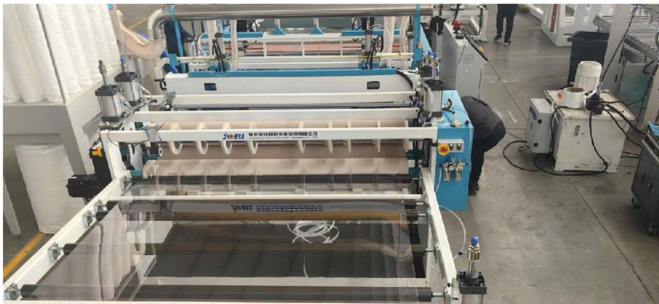
Corrugated, hollow, and solid sheet machines with widths of 1.22m, 1.56m, 2.1m, and 2.5m
